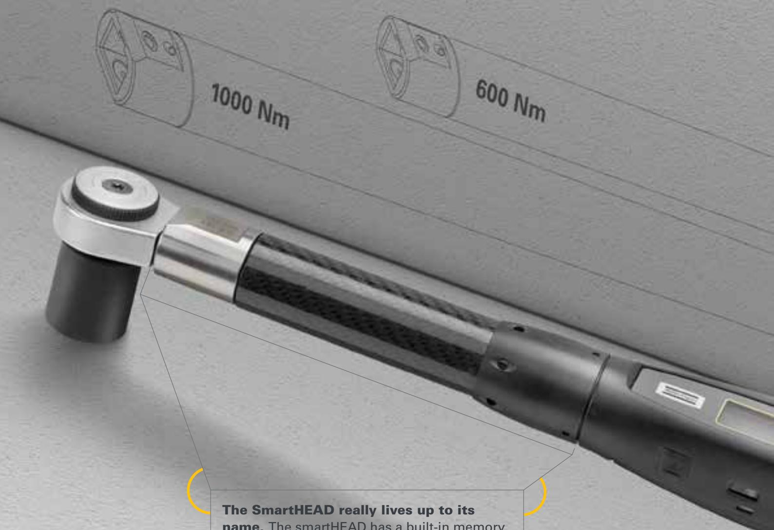
**The SmartHEAD really lives up to its name.** The smartHEAD has a built-in memory chip to store calibration values that are automatically recognized by the STwrench controller. They come in 21 different versions from 15 Nm up to 1000 Nm, with or without angle reading. The smartHEAD is fast to exchange, this makes STwrench easy to upgrade and Service.
